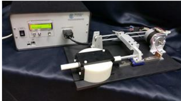
Figure 2: Photo of the switchable phantom kit.
